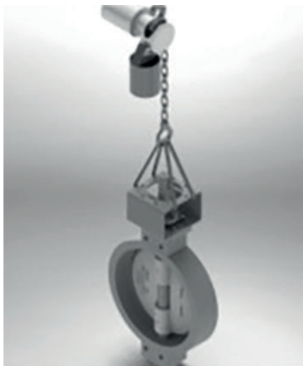
Figure 4-1: Sample lifting points for butterfly valves
