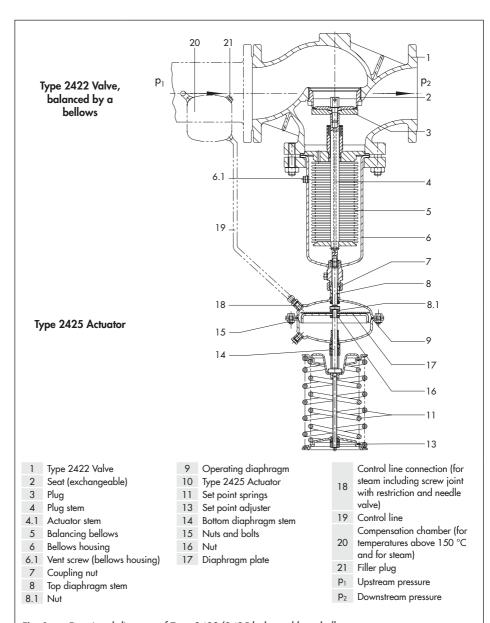
Fig. 1: Functional diagram of Type 2422/2425 balanced by a bellows
