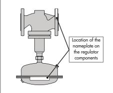
Fig. 5: Nameplates of the Type 2422 Valve and the Type 2425 Diaphragm Actuator
