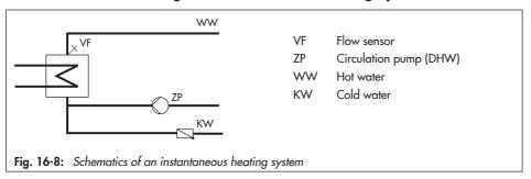
The control of the required 'DHW temperature' at the flow sensor VF is only active during times-of-use of the circulation pump ZP.
