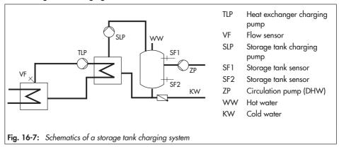
The controller begins charging the storage tank when the water temperature measured at sensor SF1 falls below the 'DHW temperature set point' by 0.1 °C. If the flow temperature in the system exceeds the desired charging temperature, the controller tries to reduce the flow temperature in the heating circuit for up to three minutes before the exchanger charging pump is activated together with the storage tank charging pump.
