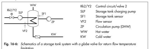
Globe valve and flow sensor VF2 are used exclusively for return flow temperature limitation in the schematics shown above. The pre-control circuit provides at least the same flow temperature as in the standard schematic version which is calculated from 'DHW temperature set point' + 'Charging temperature boost' + 'Boost set point of pre-control circuit'.
